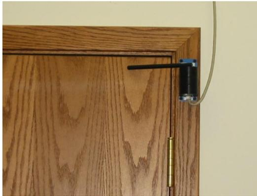
**Figure 39 –Position of Encoder on door**
